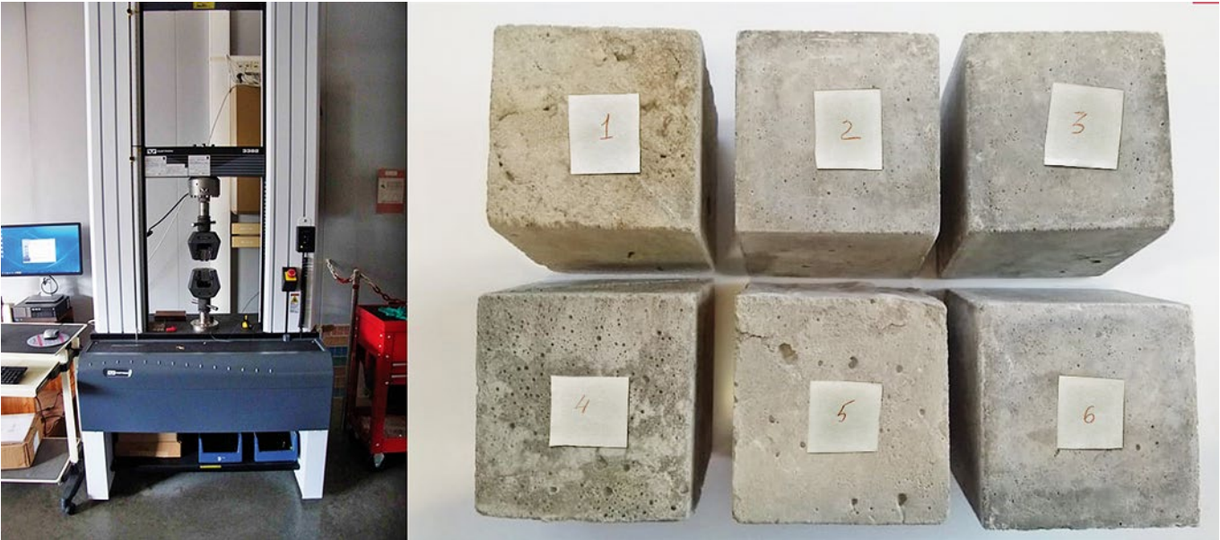
Fig. 5. Instron 1100 HDX universal testing machine and shotcrete samples for strength testing
