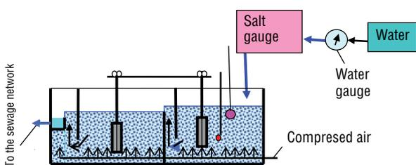
Fig. 6. Rational tank for two-stage countercurrent flushing
