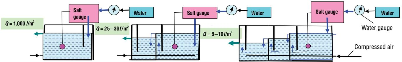
Fig. 1. Cascade flushing used to reduce the need for water per m<sup>2</sup> of coating
