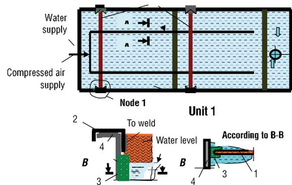
Fig. 7. Method of improving the two-stage flushing tank 1 — additional partitions; 2 — clamp for fastening the partition on the tank wall; 3 — sealing plate made of porous chemically resistant rubber; 4 — tank body; 5 — calibration valve with a reset flywheel; 6 — shut-off valve
