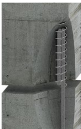
Fig. 6. Rebar lapping in grout-filled hole
