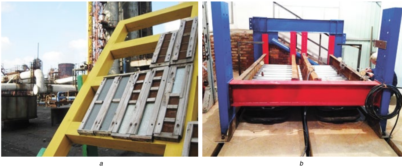
Fig. 3. Justification of LC stability indicators during definitive tests: a — bench corrosion tests; b — bench strength tests
